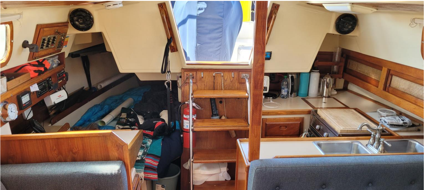
Plate 14: Interior layout of “Adventure”, looking aft, showing galley and aft quarter-berth.
