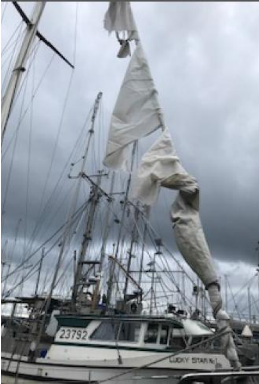
Plate 1. Headsail damage incurred from the November windstorm at the Fisherman's Wharf.
